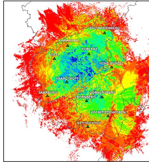
Fig. 11: Multiple coverage of all DRM+ SFNs with 16-QAM (variant PFALZ1)<sup>5</sup>
