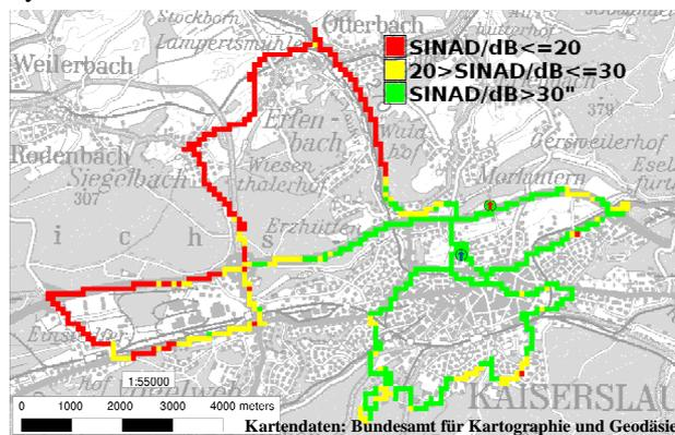
Fig. 4. Measured mobile coverage for FM with TX RB switched off. Assignment of measured coverage see Tab. 3.
