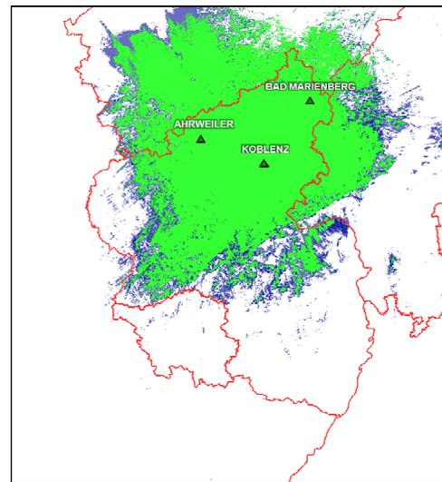
Fig. 5: DRM+ coverage of SFN KOBLENZ
