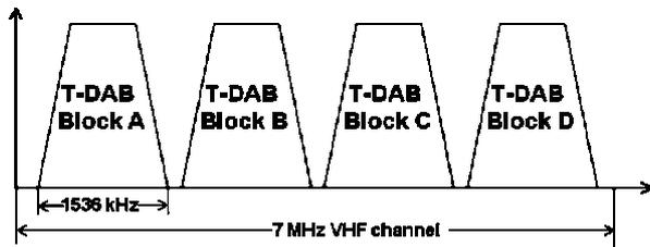
Fig. 1. T-DAB frequency blocks in VHF Band III
