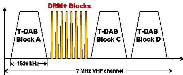
Fig. 2 DRM+ frequency blocks in a free range added to T-DAB frequency blocks in VHF Band III
